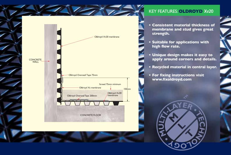
Oldroyd Xv20 is manufactured from polypropylene. Combined with a unique, temperaturecontrolled manufacturing process, this produces an exceptionally straight, durable membrane. The patented "X" pattern embossed into the membrane makes it easy to cut and fold. This quality also allows for shrinkage movements frequently encountered when screeds are applied, thus minimising potential cracking problems.
