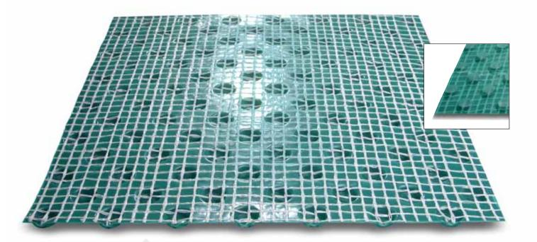
Oldroyd P is a studded polypropylene waterproofing membrane with a special mesh welded to one side. It is fixed to damp, contaminated walls using Oldroyd Plaster Plugs, with the studs facing the wall. This creates an air gap which allows the wall to breathe whilst blocking the passage of moisture. On the reverse side of the membrane the special mesh can be plastered onto, allowing a dry plaster finish to be achieved without risk of contamination from any damp or salts in the wall.
